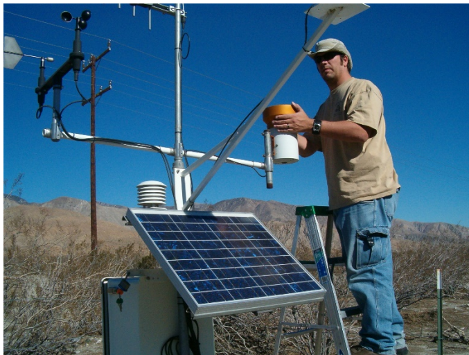
Routine maintenance of a weather station on the Morongo Indian Reservation.
